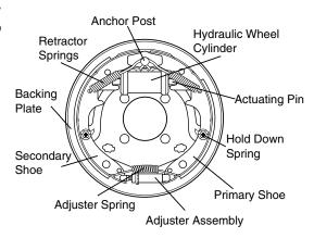
to leave the anchor and causes the primary shoe to move against the anchor. Action of the brake is the same in reverse as forward.
