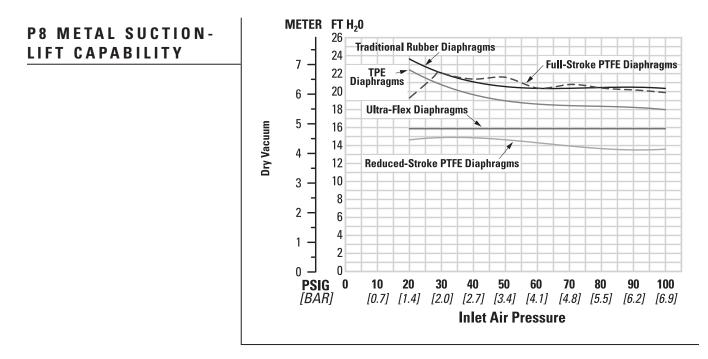
Suction-lift curves are calibrated for pumps operating at 305 m (1,000') above sea level. This chart is meant to be a guide only. There are many variables that can affect your pump's operating characteristics. The number of intake and discharge elbows, viscosity of pumping fluid, elevation (atmospheric pressure) and pipe friction loss all affect the amount of suction lift your pump will attain.
