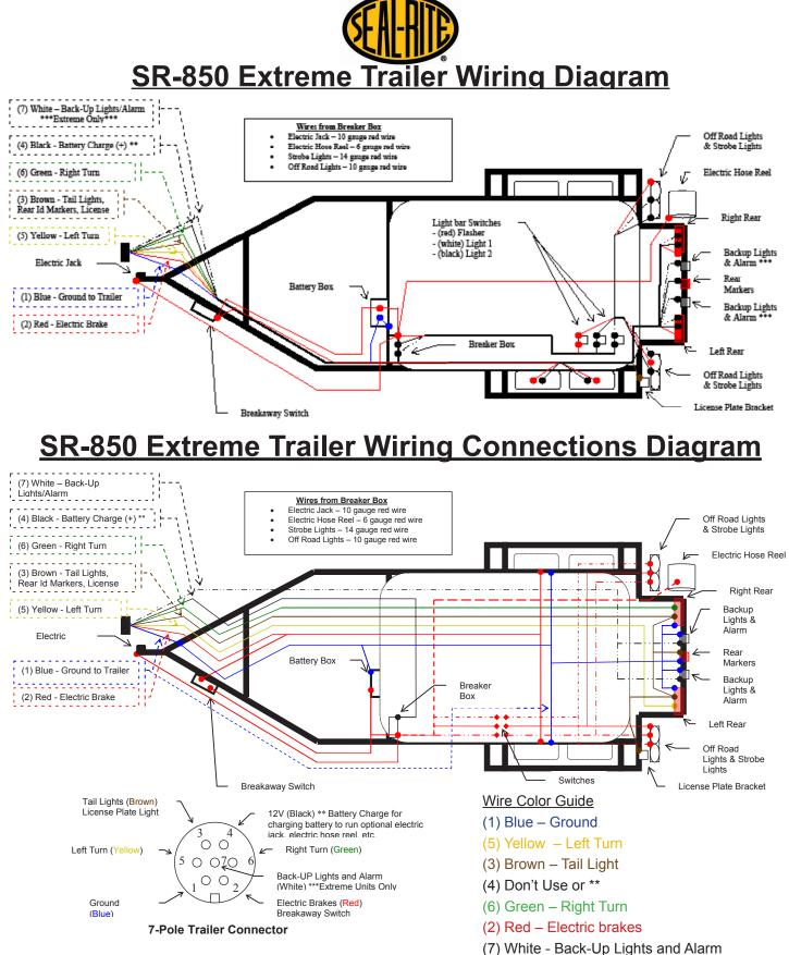
Note: The above wiring diagrams are not intended as a diagram for the wiring on the tow vehicle. It is strictly for the wiring of the Seal-Rite trailer. Tow vehicle wires should be located by function only, as color coding is not standard among all manufacturers.
