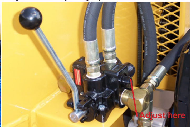
Diagram 1B - Adjusting Hydraulic Control Valve
