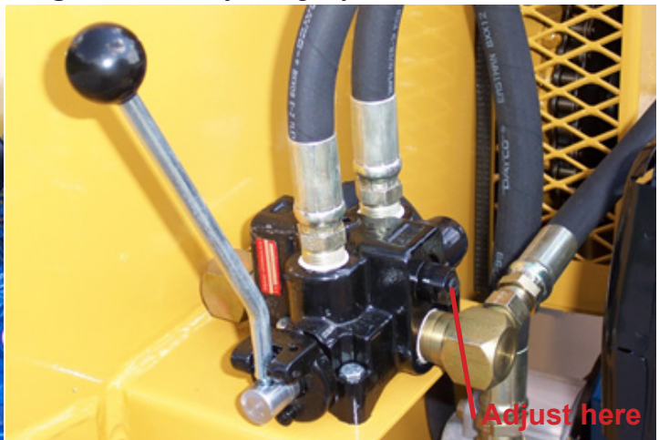
Diagram 1B - Adjusting Hydraulic Control Valve
