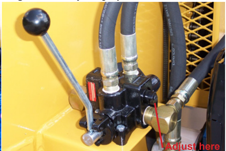
Diagram 1B - Adjusting Hydraulic Control Valve
